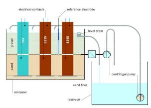
**Figure 2: Schematic of Test Setup**
