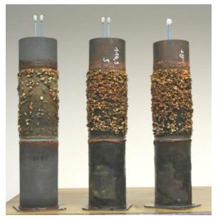
Figure 4: Picture of Samples after Testing (pre-cleaning)
