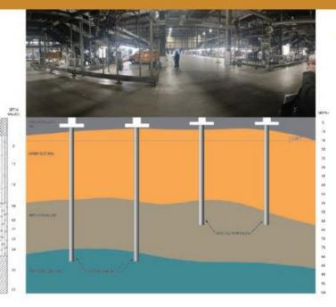
Using a design-build approach and multiple load tests performed as production progressed, the designers were able to optimize pile design lengths, capacities and reduce the number of piles to support the footings in the dense lower alluvium and the hard-residual clays.
