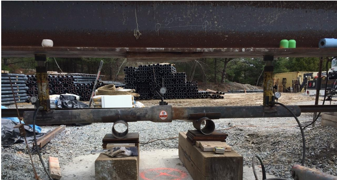
Figure 5: Ductile Iron Pile Bending Test Setup (U.S.A.)
