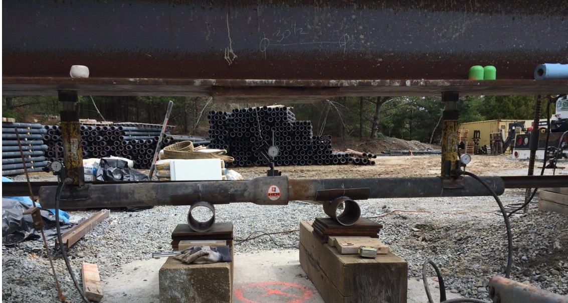
Figure 5: Ductile Iron Pile Bending Test Setup (U.S.A.)
