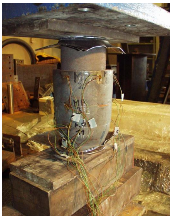
Figures 3a, b: Cross-section of Bell-Spigot Pile Socket and Laboratory Test Setup (Niederwanger and Lehar, 2001)
